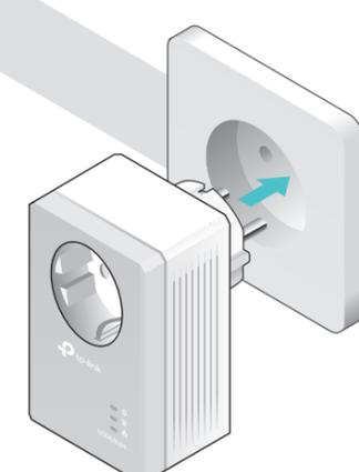
**More:** To add additional Powerline adapters and extenders with the default settings, simply plug them into the wall sockets on the same electrical circuit.
